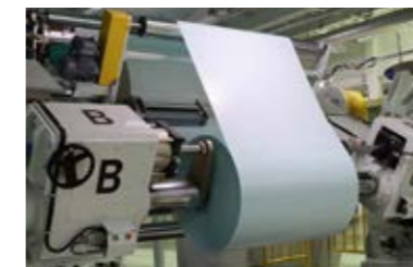
Coating equipment for solventless release paper (Kumagaya Plant)
